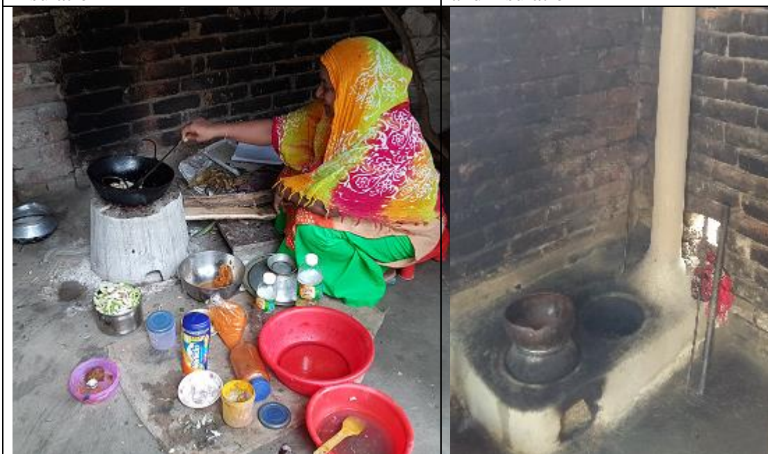
Double mouth stoves with metallic lining and insulation
