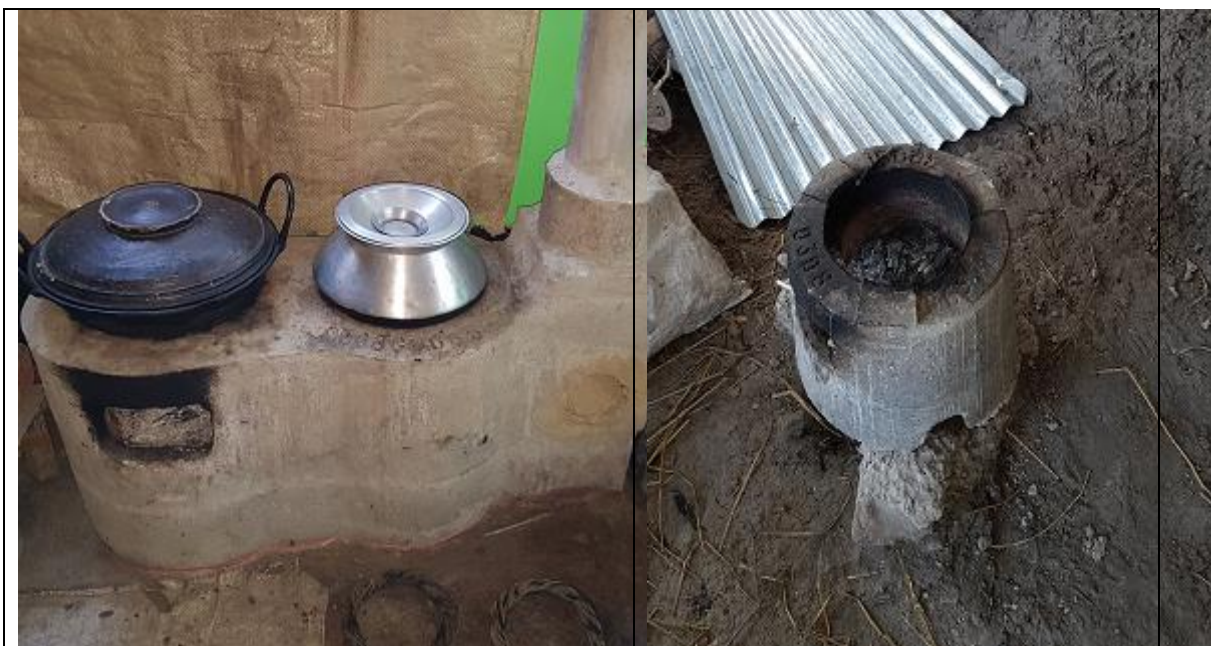
Double mouth stoves with metallic lining and insulation
