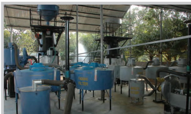
250 kW biomass gasification based power plant
