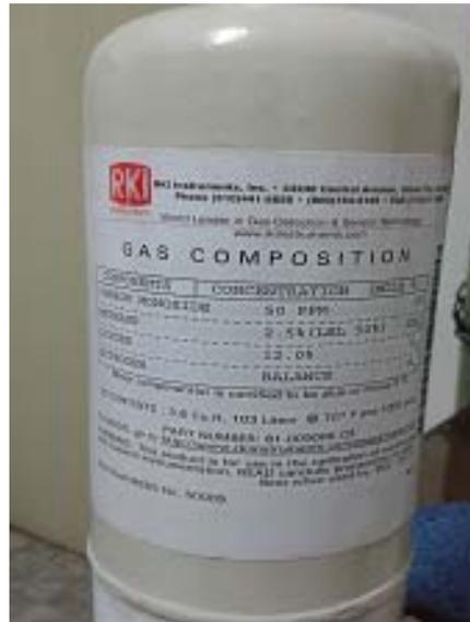
Figure 3: Calibration Gas (CO)
