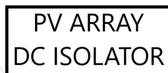
Figure 3: Sample sign required adjacent to PV array D.C. isolator / switch-disconnector
