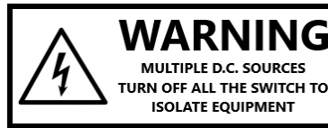
Figure 4: Sample sign required where multiple isolator / switch-disconnector devices are used
